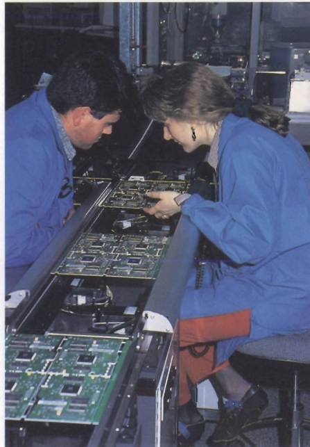
Battista Salvi (left) and Barbara Giroto inspect formatter boards on the Bergamo manufacturing line.
